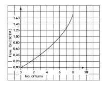
Unregulated Flow B→A with needle fully open - 107 NL/min. [3.78 SCFM] Unregulated Flow B→A with needle fully closed - 28.3 NL/min. [1.0 SCFM]
